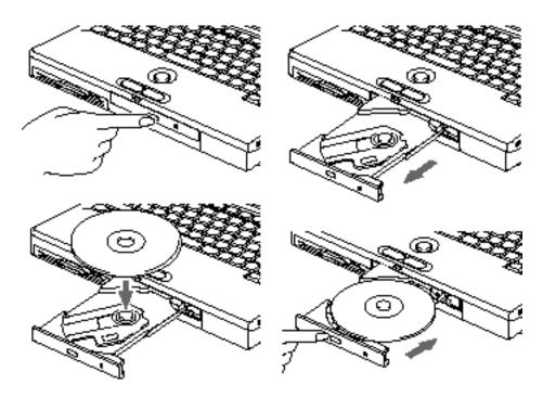
Figure 2-12 Loading/Ejecting a CD
